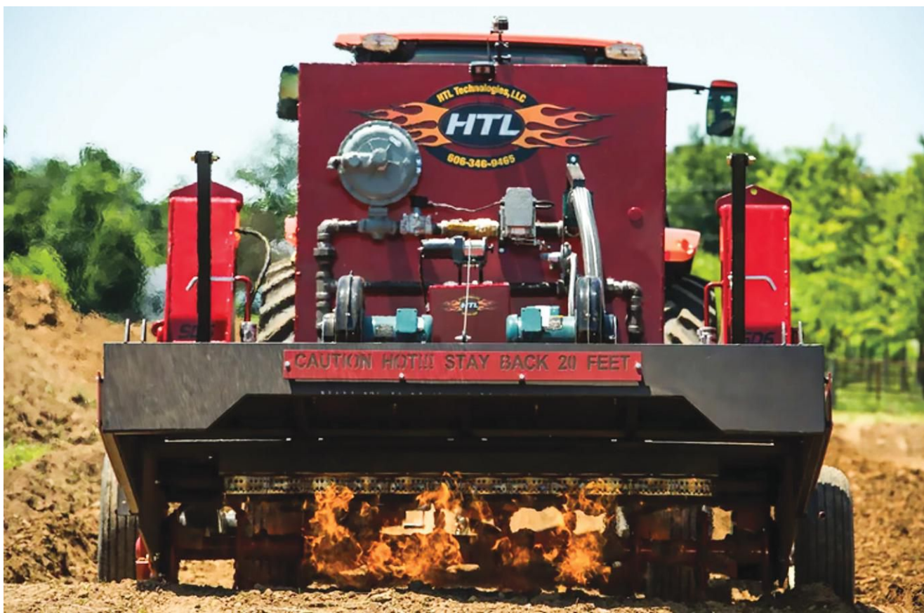
The rototiller function throws soil through the 6 million Btu flame to evaporate moisture from the soil.
