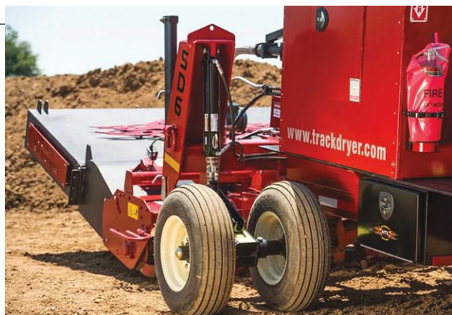
Soil dryers blow heated air through the top layers of the ground.
